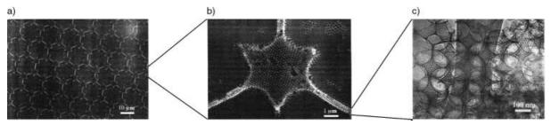
Figure 26. Electron micrographs of a structure hierarchy over three organization levels<sup>[150]</sup> prepared with the aid of microcontact printing and self-assembly: a) microcontact sample ( $d = 15 \mu m$ ), b) macroporous structure (d = 200 nm), c) mesoporous structure (d = 2 nm).
