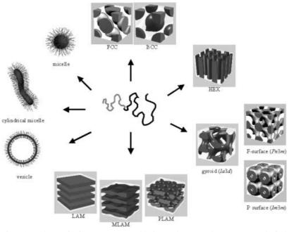
Figure 13. Self-organization structures of block copolymers and surfactants: spherical micelles, cylindrical micelles, *tcc-* and *bcc-*packed spheres (FCC, BCC), hexagonally packed cylinders (HEX), various minimal surfaces (gyroid, F surface, P surface), simple lamellae (LAM), as well as modulated and perforated lamellae (MLAM, PLAM).
