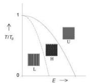
Figure 1. Transition from a disordered phase (U) to ordered phases (H, L) by variation of the temperature T and the external field E.  $T_c$  is the critical temperature above which ordered phases are not accessible. The transition  $U \rightarrow H,L$  corresponds to a self-organization.
