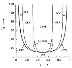
Figure 5. Theoretical phase diagram of block copolymers. Various ordered superlattices can be obtained by variation of the block lengths (*f*-axis) and the temperature ( $\chi N$ -axis; see the legend to Figure 13 for an explanation of the abbreviations). (From ref. [6].)
