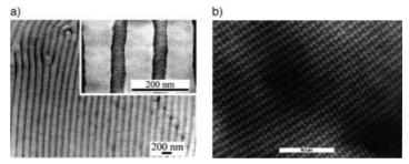
Figure 15. Complex and hierarchic superlattices of AB block copolymer/surfactant systems (a)<sup>[60]</sup> and ABC triblock copolymers (b, "knitting pattern").<sup>[61]</sup>
