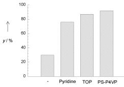
Figure 21. Percentage of reaction *y* of the Heck reaction with Pd without ligand and for different ligand systems.<sup>[114]</sup> The catalyst embedded in the micelles shows the highest reaction at considerably better stabilizing. TOP = tri-o-tolylphosphane.
