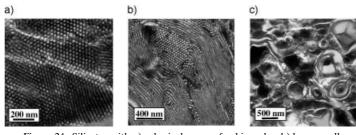
Figure 24. Silicates with a) spherical pores of cubic order, b) hexagonally ordered cylindrical pores, and c) lamellar pores prepared from lyotropic phases of block copolymers.<sup>[95, 134]</sup>
