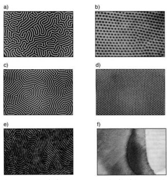
Figure 3. Lamellar (left) and hexagonal domains (right) in a ferrofluid with a) d = 1 cm, b) d = 4 µm, in a ferromagnetic film with c,d) d = 10 µm, and in a block copolymer superlattice with e) d = 40 nm, f) d = 16 nm. The examples give evidence of the universality of the order principles through pairs of forces. (From ref. [5].)
