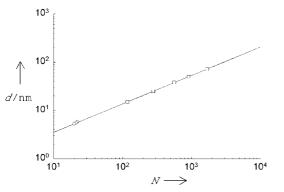
Figure 12. Long period *d* as a function of the degree of polymerization *N* of PB-PEO ( $\Box$ ) and nonionic surfactants ( $\bigcirc$ ).<sup>[50]</sup> The periodic length of the nanostructure can be specifically adjusted over the whole mesoscopic range (1–100 nm) by the degree of polymerization.
