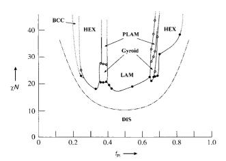
Figure 11. Experimentally determined phase diagram of PS-PI.<sup>[55, 56]</sup> The individual superlattices can be specifically prepared by adjusting the volume ratio  $f_{\rm PI}$  of the block copolymers, the total degree of polymerization N, and the temperature ( $\chi \sim 1/T$ ). The structures of the individual phases are depicted in Figure 13.
