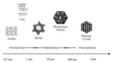
Figure 23. Typical length scales of three-dimensional porous structures.
