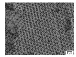
Figure 25. Photonic crystal synthesized from polystyrene latices by a sol/ gel procedure.<sup>[149]</sup>
