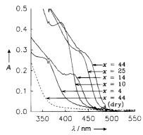
Figure 22. Blue shift of the absorption edge of CdS with decreasing particle size (size quantization effect).<sup>[115]</sup> The particle size was adjusted by the degree of polymerization x of the polymethacrylic acid block.
