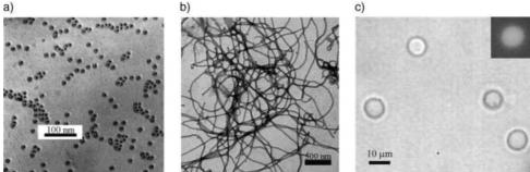
Figure 9. Electron micrographs (a, b) and optical micrographs (c) of the three most frequent forms of self-organization of block copolymers: a) spherical micelles (PS-PI/DMF),<sup>[49]</sup> b) cylindrical micelles (PB-PEO/water),<sup>[50]</sup> and c) vesicles (P2VP-PEO/water).<sup>[53]</sup> Figure c shows top right a single vesicle in which the solution of a fluorescent dye was encapsulated.
